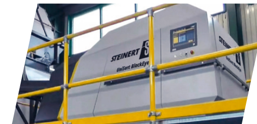
Sorting of black plastics by type using UniSort BlackEye
