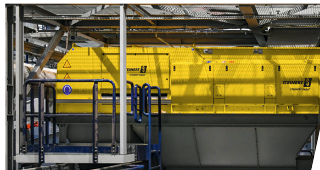
Recovery of non-ferrous metals using STEINERT EddyC
