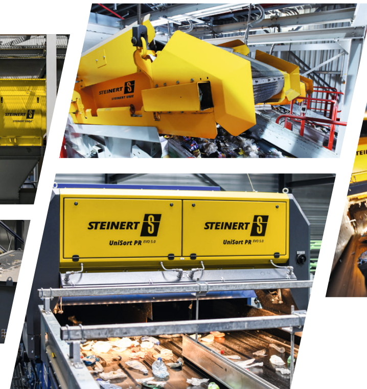
Sorting 3D recyclables using UniSort PR EVO 5.0 and AI-based sorting programs
