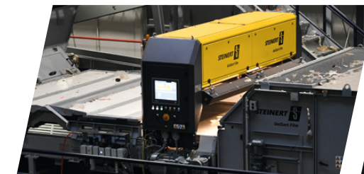
Sorting 2D plastics using UniSort Film EVO 5.0
