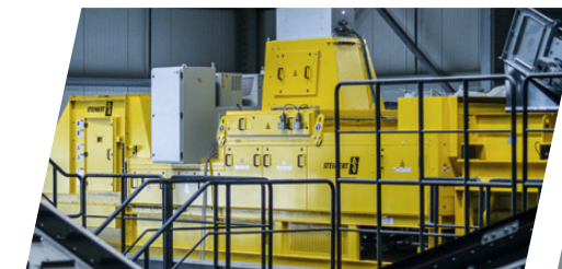
NF-metal segregation by metal type or removal of BFR plastics with STEINERT KSS | XF L
