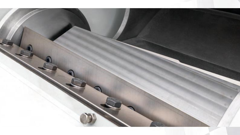
High energy-efficiency is a feature of Hellweg granulators. This is characterised by cutting rotors working according to the scissor-cut principle that have no welds, as they are produced from a solid metal blank.
