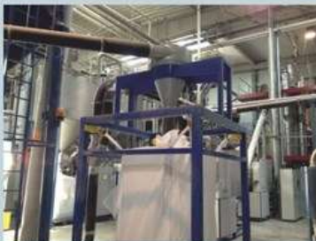
Big-bags discharge station for flakes, PET, PE, Film, PS scraps complete with discharge ampoule
