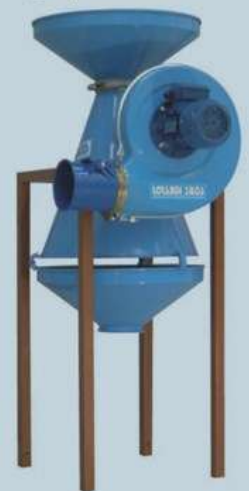
Pre-cleaner cleaning system for light parts suction
