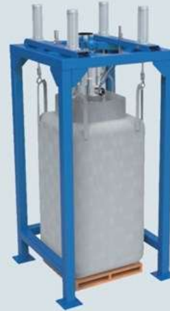
Compacting system with pistons
