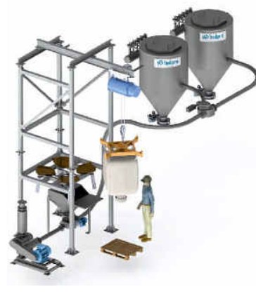
Pressure conveying system with big bag unloading
