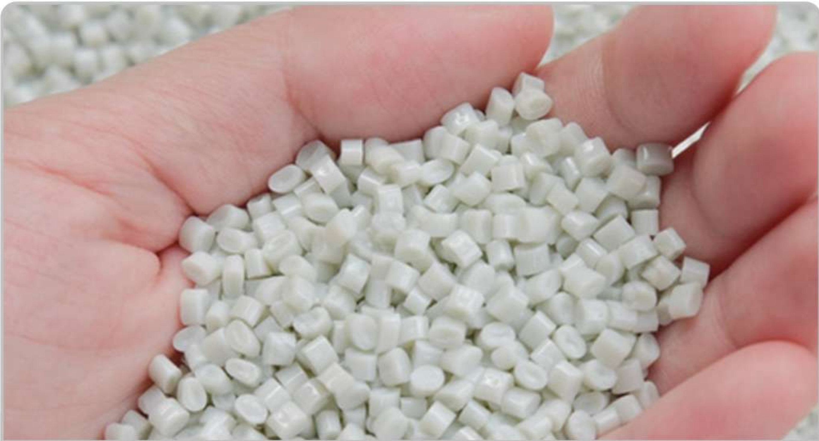
Chips for r-PET Yarns / Fibres / Technical Textiles
