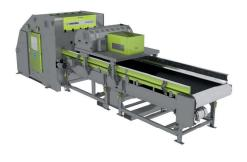
The multi-sensor sorting system VARISORT can be used universally in many different recycling applications (e.g. plastics, metal, electronic waste and solid waste recycling). It will sort mixed streams into single fractions, playing a pivotal role in ensuring the highly pure recycled material can be profitably reprocessed in the production cycle.
