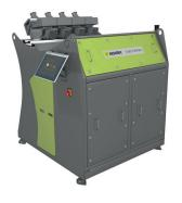
The multi-sensor sorting system FLAKE PURIFIER+ is especially designed for the operation in the plastic recycling industry. The material infeed is done by a specifically adjusted vibratory feeder. Besides the sensors for the metal and color separation, Sesotec also uses a high performance module for the recognition of contaminations (e.g. different polymer types).
