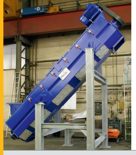
The Friction and Tornado Washers are the perfect combination for continuously cleaning heavily contaminated film and rigid plastics using water and mechanical forces. Common impurities such as
