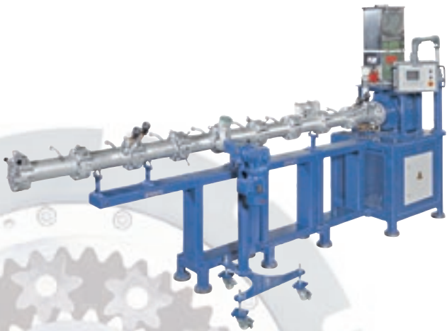
Module building block, developable up to 12 modules, 8 modules applications for the chemical and polymer industry
