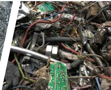
It can happen that metallic components cannot be separated into ferrous and non-ferrous fractions by the use of magnetic separators (e.g. stainless steels and composite materials). The STEINERT ISS is the logical solution to such problems.
