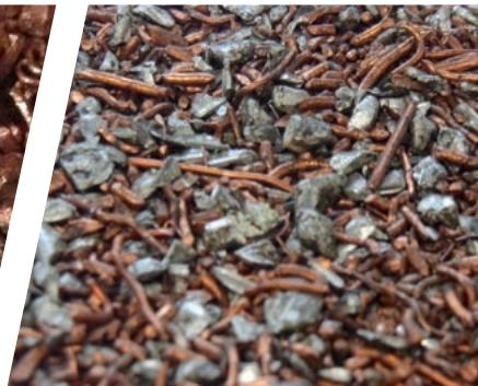
The UniSort Flake was specially developed for sorting fine bulk materials. The UniSort Flake C is ideally suited for use in metal recovery where the requirement is the cleaning of copper or aluminium strands. Extremely high levels of purity are achieved in sorting copper/aluminium. We can optionally integrate all-metal detection.
