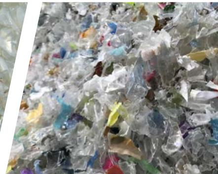
The UniSort Flake has been specially developed for sorting fine bulk materials such as plastic mixtures. The unit is fitted with a high-resolution NIR sensor and optional with all-metal sensor.
