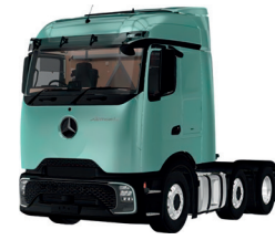
Air deflectors and cabside deflectors painted
