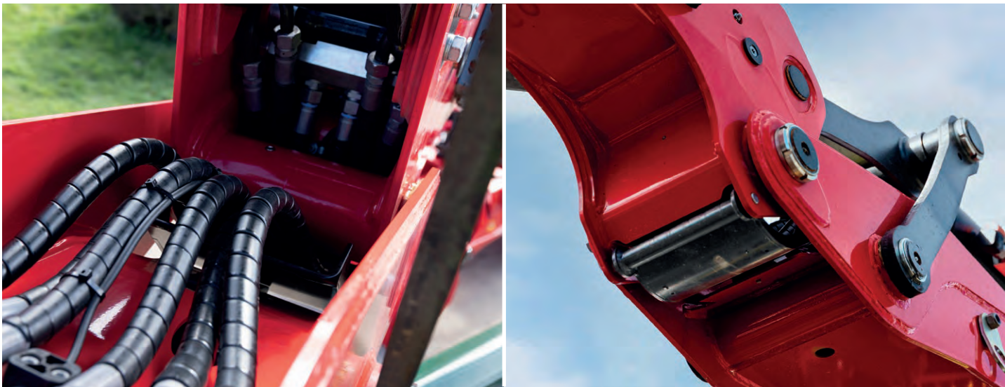
Main Boom - Knuckle Boom Transition
