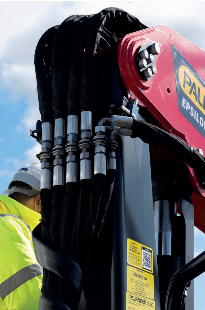
Compact Hose Package on the Column
