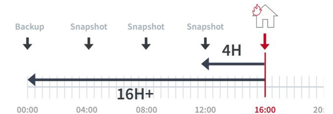
Figure 4. Though snapshots shorten RPO, they are usually taken every 4 or 8 hours (because otherwise they will have too much impact on the performance and use too much disk space). This results in a better RPO than a traditional backup, but up to 4 or 8 hours of work can be lost when an incident occurs.
