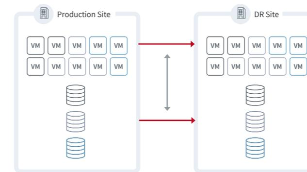
**Figure 1.** Array-based and appliance-based replication requires coordinating two replication products, both for the physical and the virtualized environment. This increases management complexity and undermines the investment made in virtualization.
