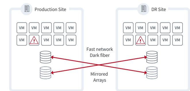
**Figure 2.** By mirroring systems over a fast network a very high availability is possible, but corrupted software components are replicated as well.
