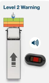
If a VRU is detected in any zone when the vehicle begins to move off, the display will alert the driver with a red light and acoustic alarm.
