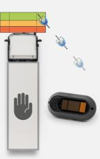
When stationary, a light is shown in the relevant left or right zone if a moving VRU is detected.
