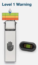
When stationary, a light is shown if there is a static or moving VRU in the middle detection zone.
