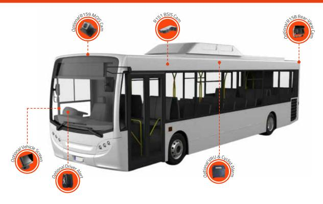
The system eliminates all vehicle blind spots, warning the driver and VRUs of imminent danger through an audible and visual alert.
