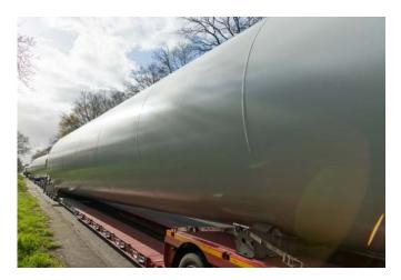
For most elastic materials, a weight load of 630 tons per square metre is a very unreasonable demand. But not for our **REGUPOL cargo mat 1000**°. Heavy loads can be secured safely and reliably, without causing any inadmissible deformation of the mat that might compromise the safety of the heavy objects or materials being transported.
