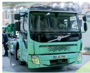
**ELECTRIC LAUNCH: Volvo** Trucks used the expo as the UK launchpad for its new FE-Electric, designed for zero-emission refuse collection and urban distribution duties. The 26/27-tonne chassis cab has a range of up to 200km and produces zero tailpipe emissions. Compared with a conventional refuse collection vehicle, which Volvo said can emit approximately 31,300kg of CO2 in tailpipe emissions a year, the FE-Electric emits nothing and lasts for up to 10 hours.
