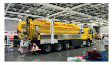
Volvo FM 8x4 tridem chassis with a triple rear bogie that uses a steering and lifting front axle to maximise manoeuvrability.
