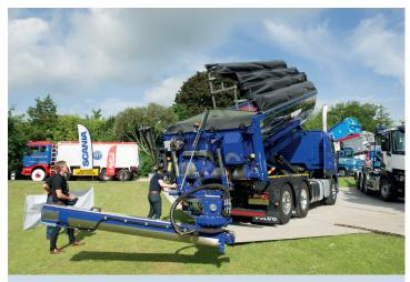
**SAFETY FIRST:** While the road transport world ponders driverless trucks, the Swedish ReCoDrive system, as fitted to a 6x2 Volvo FE with a Sprider asphalt patching machine, already allows the operator to safely move the truck from a remote control while operating the equipment. It allows the operator to lay up to 60 tonnes of asphalt in a day helped by its body, which is insulated to Scandinavian standards. The system is sold in the UK by Plant Supply of Hirwaun, south Wales.
